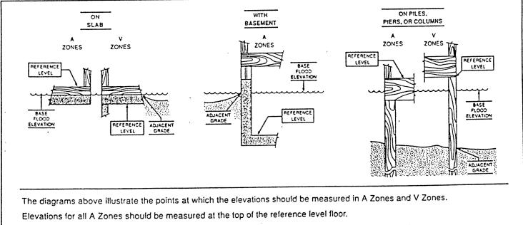
Elevations for all V Zones should be measured at the bottom of the lowest horizontal structural member.
