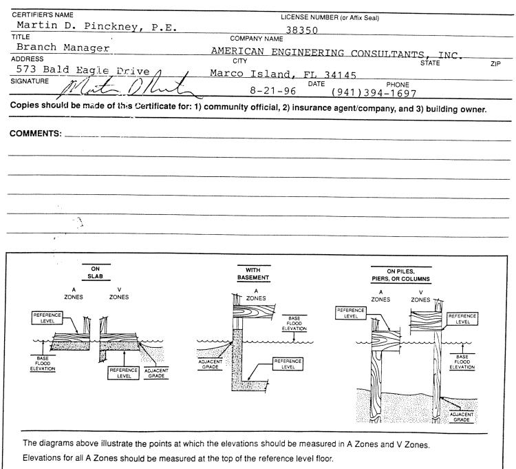
Elevations for all V Zones should be measured at the bottom of the lowest horizontal structural member.
