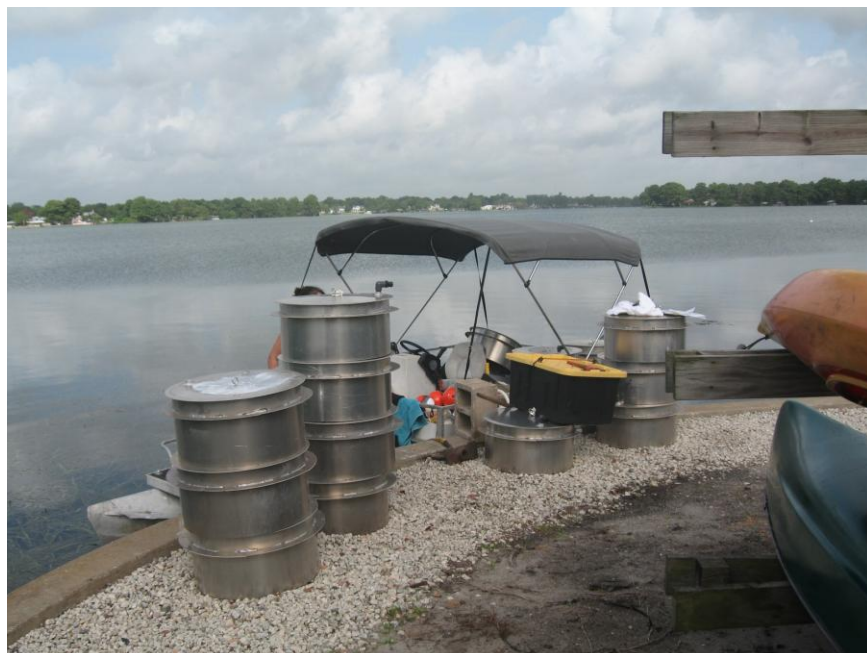
Figure 4-6. Seepage Meters Being Prepared for Installation.
