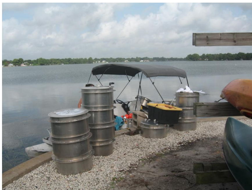
Figure 4-6. Seepage Meters Being Prepared for Installation.
