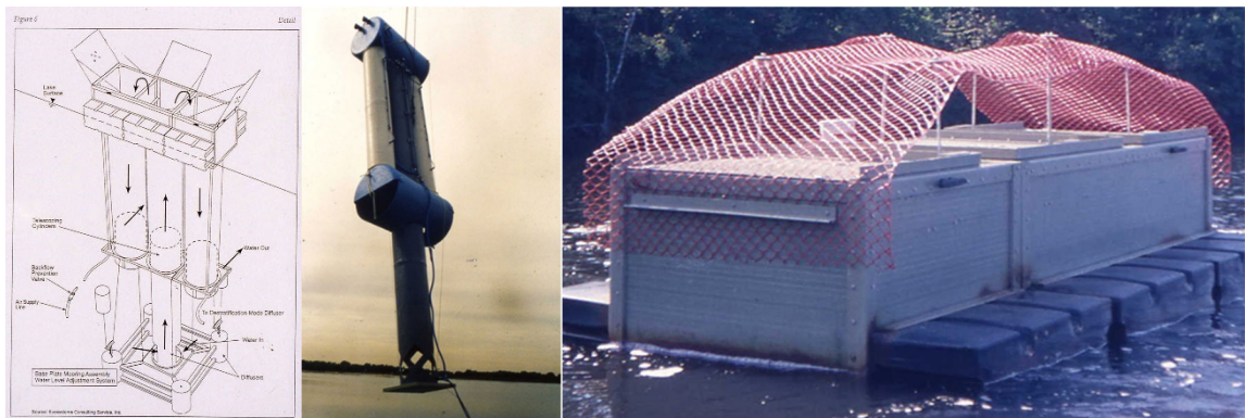
Figure 1: Example of Air-lift aerators showing schematic (left), install (middle), and operation (right).
